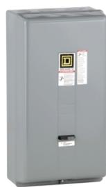
NEMA Motor Starter, Type S, nonreversing, Size 3, 90A, 50 HP at 460 VAC, 5 kA SCCR, 3 phase, 3 pole, melting alloy, 208 VAC coil, NEMA 1 [TAA]
