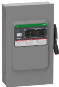
**Safety switch, heavy duty, fused, viewing window, Type 1, 240V, 200A, 3 pole, neutral installed**
