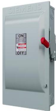
Siemens Low Voltage Circuit Protection Heavy Duty Safety Switch. 3-Pole 3-Fuse and solid neutral Fused in a type 1 enclosure (indoor). Rated 600VAC (200A).
