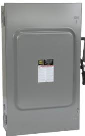
Safety switch, general duty, fusible, 3 pole, 4 wire, 240VAC, 200A, Type 1, with neutral
