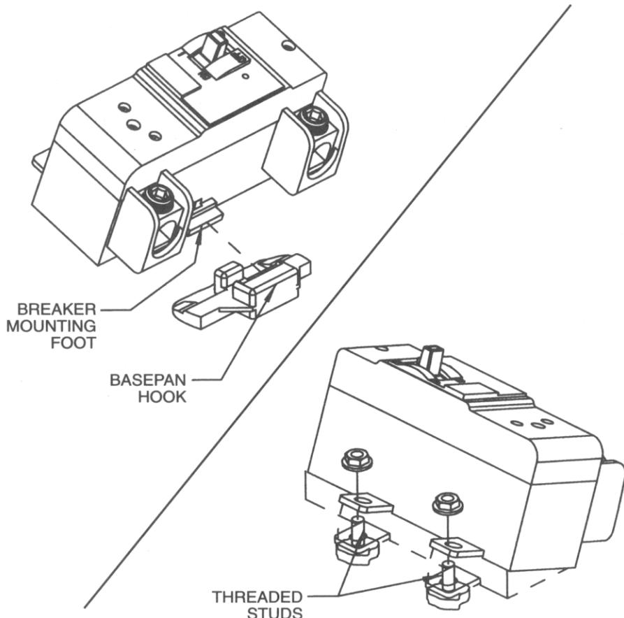
TO INSTALL, REMOVE CONNECTORS FROM LOAD CENTER. INSERT THE BREAKER FOOT INTO THE BASEPAN HOOK AS SHOWN. ROTATE THE BREAKER ALLOWING THE (2) THREADED STUDS TO PASS THROUGH THE TERMINAL SLOTS. ATTACH USING THE TWO HEX NUTS AND TORQUE TO 50 LB-IN.
