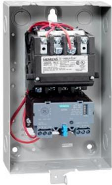
Non-reversing motor starter, Size 00, Three phase full voltage, Solid-state overload relay, OLR amp range 3-12A, 110V 50Hz / 120V 60Hz coil, Non-combination type, Enclosure type 1, Indoor general purpose use, Standard width enclosure
