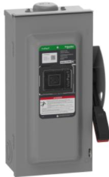
**Safety switch, heavy duty, fused, viewing window, NEMA 3R, 240V, 60A, 3 pole, neutral installed**
