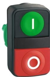
Head for double headed push button, Harmony XB5, 1 green flush, 1 red projecting, 22mm, spring return, unmarked
