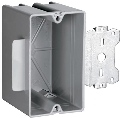
Single gang, wood and steel stud bracket box with 3/8 offset for wood and steel stud mounting. It has two Quick/Click Entries for each end, for use with 3/8 and 5/8 wallboard. It is available in single, two, three, four gang and 4 inch square boxes. It is m
