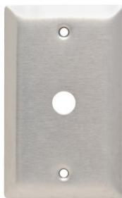
Single-Gang, Single telephone or cable outlet with removable 13/32 ft ID grommet in 17/32-inch hole. Smooth 302/304 stainless steel.
