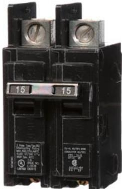
Siemens Low Voltage Molded Case Circuit Breakers General Purpose MCCBs - Type BQ, 2-Pole, 120/240VAC are Circuit Protection Molded Case Circuit Breakers. 2-Pole Common-Trip circuit breaker type BQ. Rated 120/240V (015A) (AIR 10 kA). Special features: line side lugs included. Note: Load side lugs are included.
