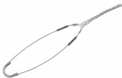
FC52: Bus Drop, Closed Mesh, Single Eye, Cable Diameter 0.53 - 0.73 inches, Bale Length 9-in, Mesh Length 6.5-in, Break Strength 1100 lbs.
