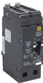
Mini circuit breaker, E-Frame, 20A, 2 pole, 600Y/347VAC, 25kA max, bolt on [TAA]
