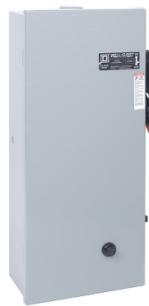
Pump Panel, NEMA Type S, Well Guard, Size 1, 27A, 10HP, 5kA SSCR, 30A fuse clip, Motor Logic SSOLR, 110/120VAC 50/60Hz coil, NEMA 3R
