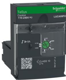
Standard control unit, TeSys Ultra, 3P, 0.15 to 0.6A, 690VAC, thermal magnetic protection, class 10, 110 to 240VAC/DC coil
