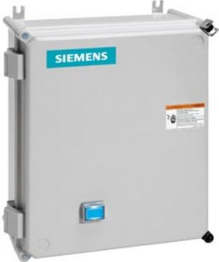
Non-reversing motor starter, Size 2, Three phase full voltage, Solid-state overload relay, OLR amp range 13-52A, 110V 50Hz / 120V 60Hz coil, Non-combination type, Enclosure type 4X fiberglass, Water/dust tight noncorrosive, Standard width enclosure
