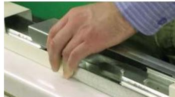
3. Tighten the two screws on the internal clip.
