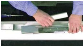
2. Slide the two pole sections together.
