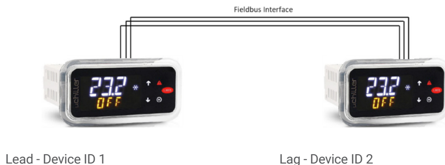
Figure 4 Lead-Lag network connectivity
