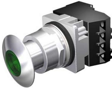
30mm Command/52, Chrome Finish Heavy Duty, Watertight/Oiltight Complete Metal Unit Illuminated Push-Pull Operator Full Voltage, 120V AC/DC LED Lamp Mushroom Head Cap Small 1 3/4" (44.5 mm) Metal, Chrome with Green Lens 2 Position Maintained, Pull-to-Release with 1 N.O. - 1 N.C. Heavy Duty Contacts, A600/P600 UL Listed, CSA Certified NEMA 1,3,3R,4,4X,12,13 & Automotive Standards
