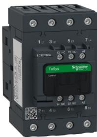
IEC contactor, TeSys Deca, nonreversing, 80A resistive, 4 pole, 4 NO, 110VAC 50/60Hz coil, open style
