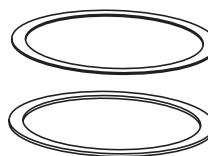
**Tile Shim -** Used for floor coverings greater than 3/16" (4.8mm). The 6TS will allow the top surface of the cover to be flush with the finished floor. Includes: six (6) 1/16" (1.6mm) thick shims. Up to a total of 3/8" (9.5mm) of adjustment.
