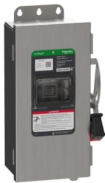
**Safety switch, heavy duty, fused, viewing window, Type 4X, 600V, 30A, 3 pole, ground lugs**
