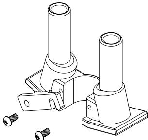
**Step 3.** Thread 1/2" trade size conduit into COM50 Communication Adapter, or 3/4" trade size conduit fitting into COM75 Communication Adapter.
