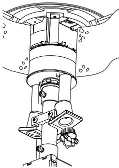
**Step 4.** Attach conduit to fitting and pull wire or cable through raceway.
