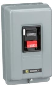
Manual starter, integral horsepower, NEMA M1, 600VAC, 3 pole, 10HP at 380/575VAC, 3 phase, no indicator, NEMA 1
