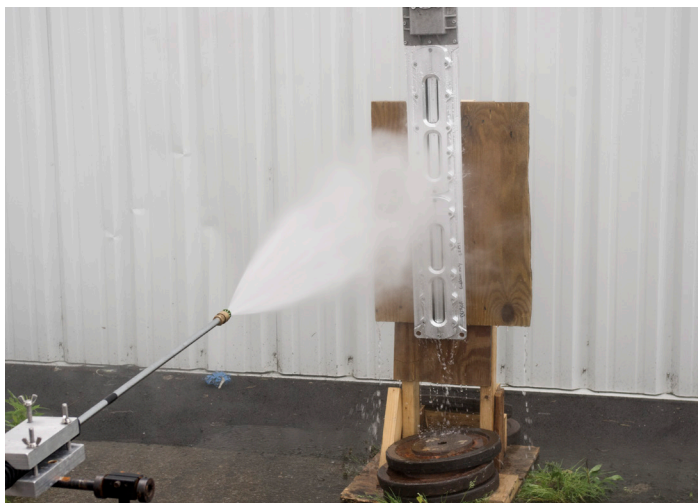
XPLA tested to withstand 2,000 psi hose test at 5 ft. distance
