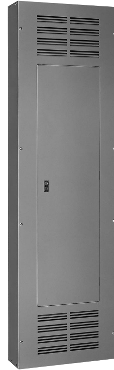
NEMA 1 Enclosure with Vented Hinged Trim Front with 3 Point Latch (required if 175 A or 200 A QO(VH) circuit breakers are installed)
