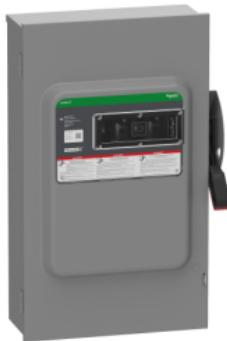
**Safety switch, heavy duty, fused, viewing window, NEMA 3R, 240V, 200A, 2 pole, neutral installed**
