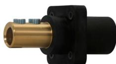
Eaton Crouse-Hinds series Cam-Lok J Series E1016 insulated receptacle, Up to 400A continuous, 1/0-4/0 AWG, Black, Double set screw, Female, Thermoplastic elastomer (TPE), 600 Vac/dc
