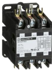
Contactor, Definite Purpose, 60A, 3 pole, 30HP at 575VAC, 3 phase, 24/24VAC 50/60Hz coil, open
