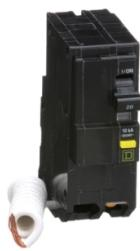
Mini circuit breaker, QO, 20A, 2 pole, 120/240VAC, 10kA, plug in, 6mA grd fault A, pigtail [TAA]
