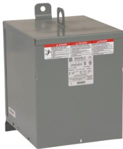
Transformer, dry type, encapsulated, 5kVA, 1 phase, 480V primary, 120/240V secondary, 13B, 115C rise [TAA]
