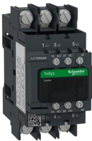
IEC contactor, TeSys Deca, nonreversing, 65A, 40HP at 480VAC, 3 phase, 3 pole, 3 NO, 230VAC 50/60Hz coil, open style
