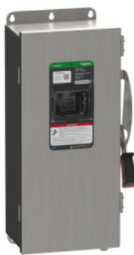
**Safety switch, heavy duty, fused, viewing window, Type 4X, 600V, 100A, 3 pole, ground lugs**
