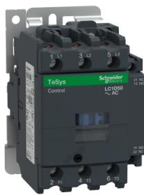
IEC contactor, TeSys D, nonreversing, 50A, 40HP at 480VAC, up to 100kA SCCR, 3 phase, 3 NO, 120VAC 50/60Hz coil, open
