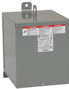
Transformer, dry type, encapsulated, 10kVA, 1 phase, 480V primary, 120/240V secondary, 13B, 115C rise [TAA]
