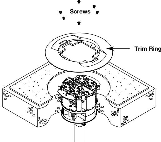
**Step 4.** Pull receptacles and receptacle brackets out of Poke-Thru device.
