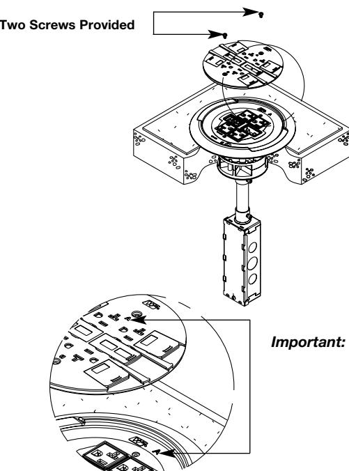
**Important:** Letter indicators need to be lined up for correct circuit identification.
