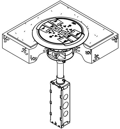
**NOTE:** Factory supplied junction box shown. Junction boxes must be located in an accessible location. Poke-Thru devices with an "LJB" or "LJB25" suffix are supplied without a junction box (supplied by others).
