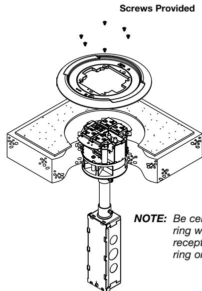
**Step 7.** Place gasket support on receptacle bracket. Place internal gasket on gasket support and press around edge to seat the gasket into the groove in the trim ring.
