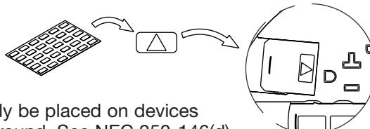
**NOTE:** The orange triangle shall only be placed on devices that are wired for isolated ground. See NEC 250-146(d).
