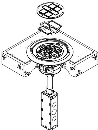
**Step 8.** Place slide holder on assembly, lining up the "A" and "B" indicators on the trim ring and the slide holder. Fasten with two screws provided.
