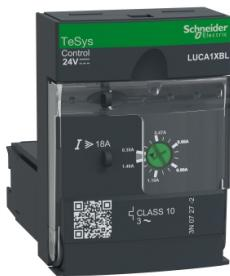
Standard control unit, TeSys Ultra, 0.35A to 1.4A, 3P motors, thermal magnetic protection, class 10, coil 24VDC
