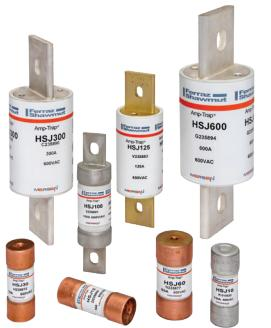
The High Speed J (HSJ) fuse combines the low  $I^2t$  of a semiconductor fuse and the branch circuit performance of a Class J UL listed fuse. This fuse was designed for the starting characteristics of solid state motor controllers. The HSJ can provide branch circuit protection per NEC requirements, as well as very low  $I^2t$  for protection of power semiconductors such as Diodes, SCRs, GTOs and SSRs.
