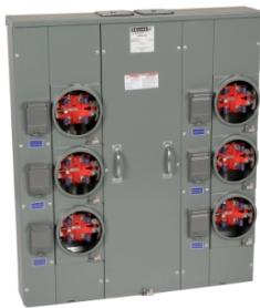
Meter center, MP Meter-Pak, 6 sockets, no bypass, 5 jaws, 600A bus, 125A max breaker rating, ringless
