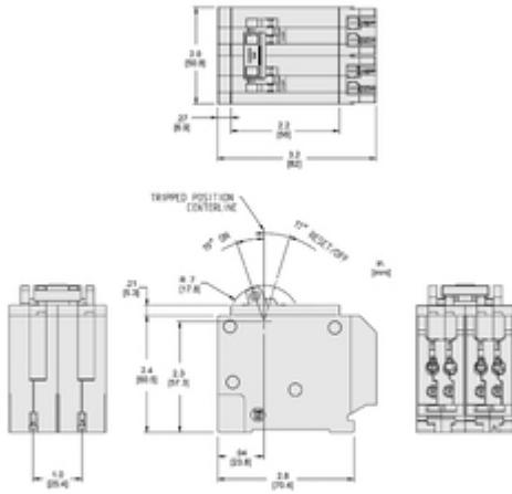
HOMT Quad Tandem Circuit Breaker. Two spaces required.
