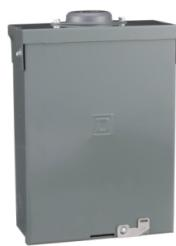
Load center, QO, 1 phase, 8 spaces, 16 circuits, 100A fixed main lugs, NEMA3R
