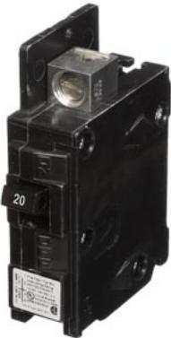
Siemens Low Voltage Molded Case Circuit Breakers General Purpose MCCBs are Circuit Protection Molded Case Circuit Breakers. 1-Pole circuit breaker type BQ. Rated 120V (020A) (AIR 10 kA). Special features: line side lugs included. Note: Load side lugs are included.
