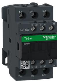
IEC contactor, TeSys Deca, nonreversing, 32A, 20HP at 480VAC, up to 100kA SCCR, 3 phase, 3 NO, 230VAC 50/60Hz coil, open
