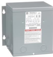
Transformer, dry type, encapsulated, 1.5kVA, 1 phase, 240x480V primary, 120/240V secondary, 8A, 115C rise [TAA]
