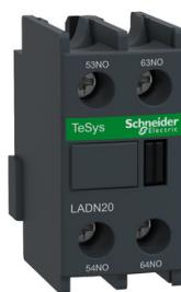
TeSys Deca, auxiliary contact block, 2 NO, top mount, screw clamp terminals, for LC1D09 to LC1D150 contactors
