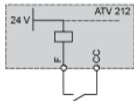
“PLC” position with PLC transistor outputs
