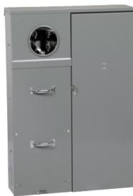
All in one, Homeline, CSED, ringed socket, 400A, surface/semi mount, 30 spaces, 40 circuits, 25kA SCCR, no bypass
