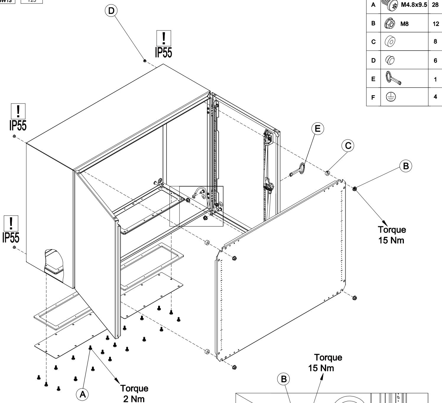
**WARNING:** When mounting on or over a combustible surface, a floor plate of at least 1.43 mm galvanized or 1.6 mm uncoated steel extended at least 150 mm beyond the equipment on all sides must be installed.
