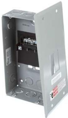
Siemens Energy Management Residential Specialty Load Centers: Small Circuit (2-10). Sub Brand: Load Centers Type: 1: Application: Residential: Voltage Rating: 120/240V Amperage Rating: 60A Phase: 1PH Load Regulation: 60A Wiring Configuration: 3w Bus Rating: 60A Interrupt Rating: 100000AIC. EQ LC 2S 4C ML 60A N1-F
