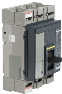
Circuit breaker, PowerPacT P, 800A, 3 pole, 600VAC, 18kA, lugs, Micrologic 5.0, 100%
